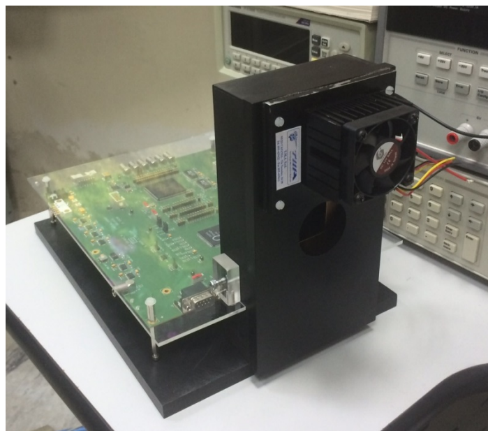
Figure 2. Citiroc evaluation board and the black light-tight box with cooling system based on Peltier TEC.
